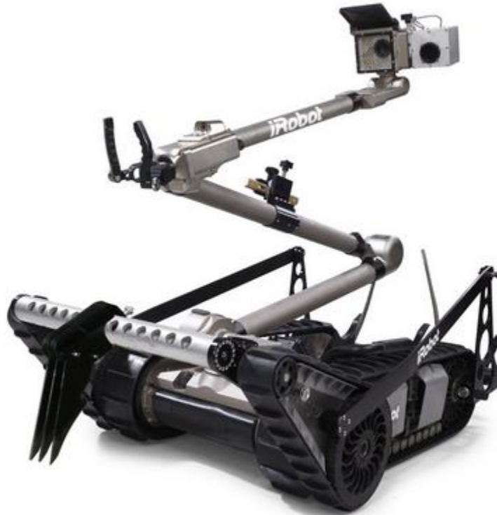
Figure 2.2 iRobot's PackBot is a good example of a traditional mobile robot that has a low center of mass and a large footprint [17]
