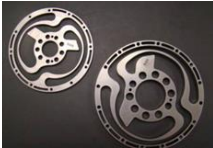
Figure 2.9 Springs used in Robonaut 2's SEAs [15]
